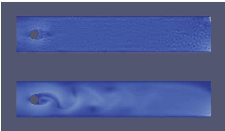
Simulated flow around an Island for SWE, Velocity Top: P_1 - P_1 , Bottom: cG(1)cG(1)
