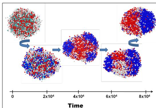
*Evolution of 3-phase particle morphology predicted by computer simulation*
