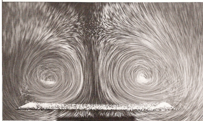
90. Vortices above an inclined triangular wing. Lines of colored fluid in water show the symmetrical pair of vortices behind a thin wing of 15^\circ semi-vertex angle at 20^\circ angle of attack. The Reynolds number is 20,000 based on
